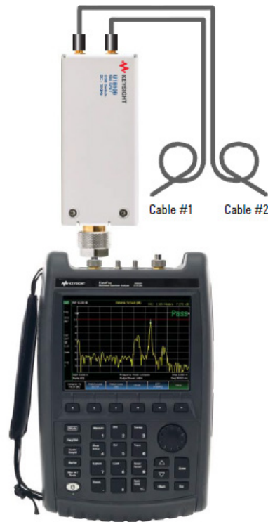
Figure 5. A single USB switch unit is a useful and time-saving addition to a field measurement kit.
